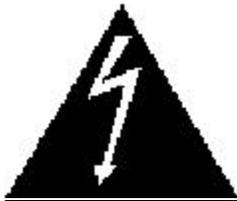
This symbol means that dangerous voltage levels are present within the equipment. These voltages are not insulated, and may be of sufficient strength to cause bodily injury if touched. The symbol may also appear on schematics.
